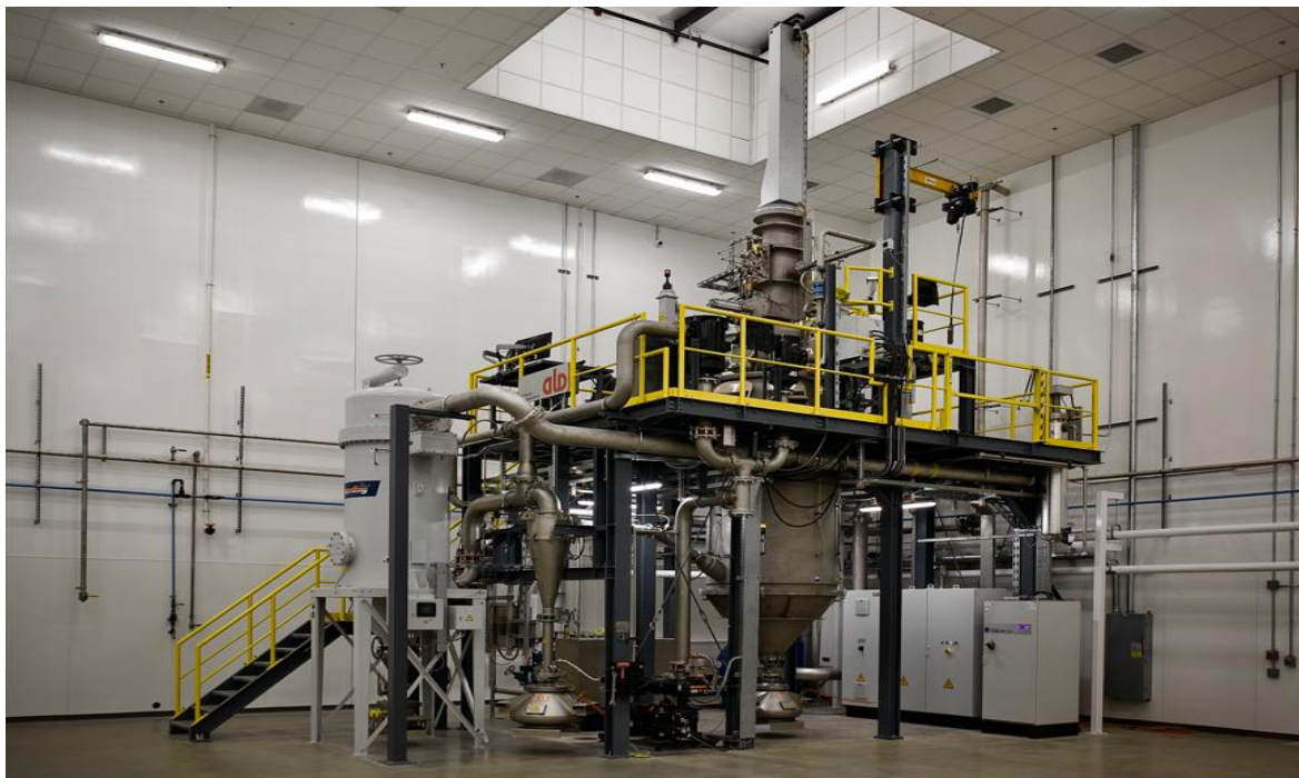
Figure 3: One of Amaero's premium EIGA atomisation systems
