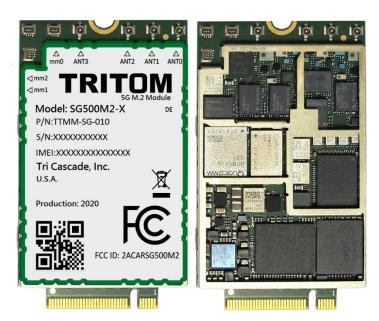
Tri Cascade's TRITOM SG500M2-X is a 5G module designed with M.2 form factor, which especially optimizes eMBB & IoT applications. Based on Qualcomm's commercial 5G platform, TRITOM SG500M2-X supports both 5G Non-Standalone (NSA) or Standalone (SA) network architectures and has fully passed T-Mobile's tests. Soon it will be able to fully support Citizens Broadband Radio Service (CBRS) for Private Networks, coupled with integrated GNSS for location service as well.
