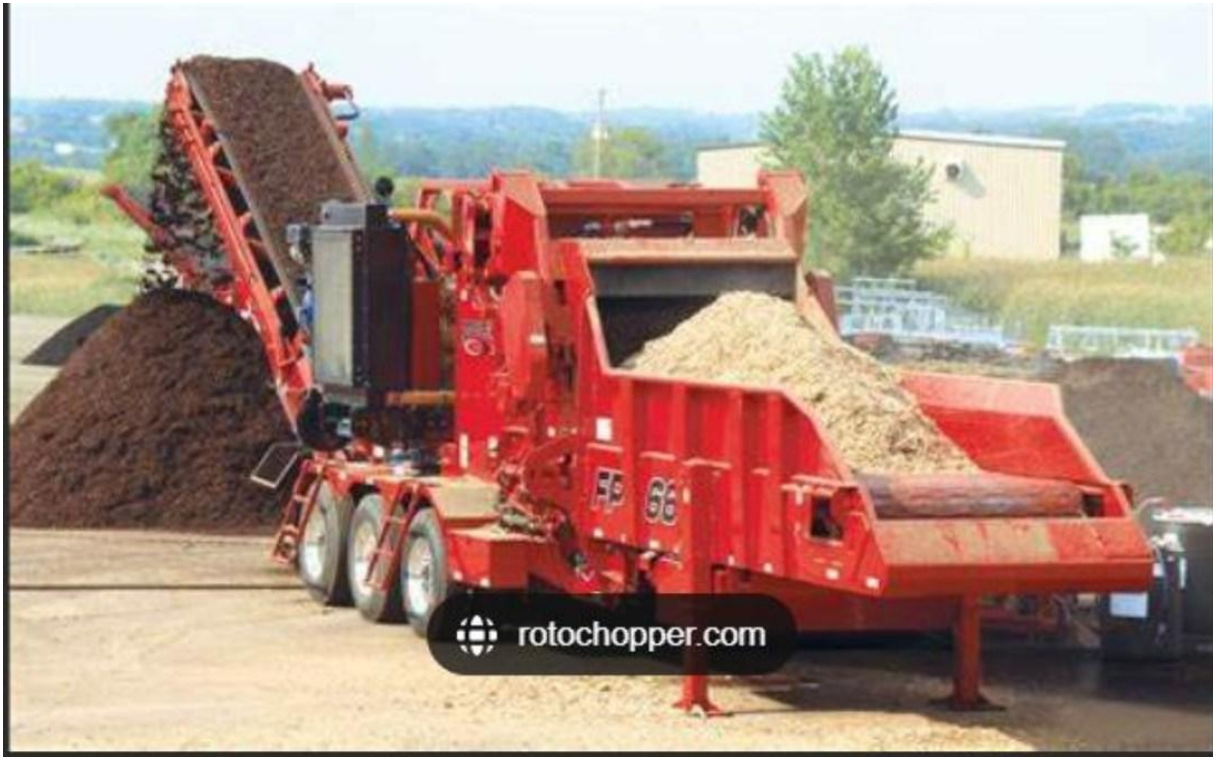
(image) A Rotochopper CP-118 mobile wood chip processor similar to the unit Santana Equestrian is acquiring. The CP-118 can grind and color wood chips into premium mulch in a single pass (Mobile Wood Chip & Mulch Processor + Colorizer Machine |Rotochopper® CP-118).
