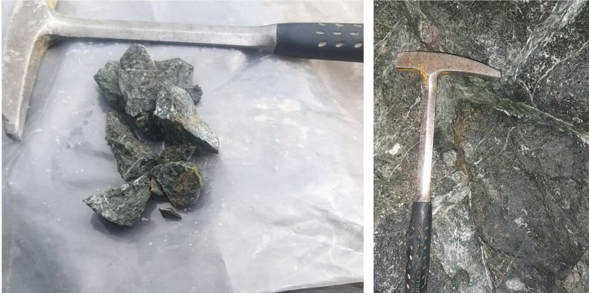
LEFT: Hand specimen samples of metapyroxenite with visible gold. RIGHT: In-situ exposure of the metapyroxenite in the prospect drive
