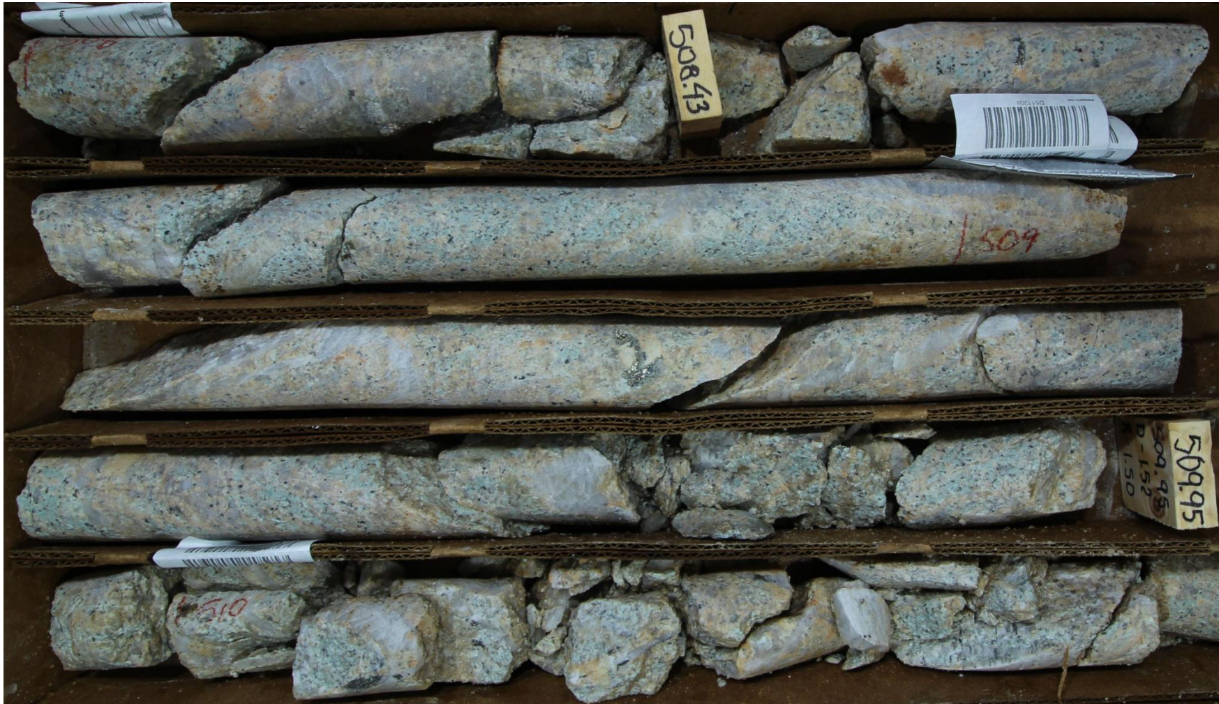
Photo 3. A second porphyry phase is predominant in the lower half of Hole 001. It is distinguished by 1-2mm, dark biotite phenocrysts showing local “shreddy” alteration ( Hole 001; 509 m; NQ ). Pyrite, chalcopyrite and molybdenite are disseminated throughout this porphyry phase and occur within 1 cm thick potassium feldspar alteration selvages to quartz “A-veins”.
