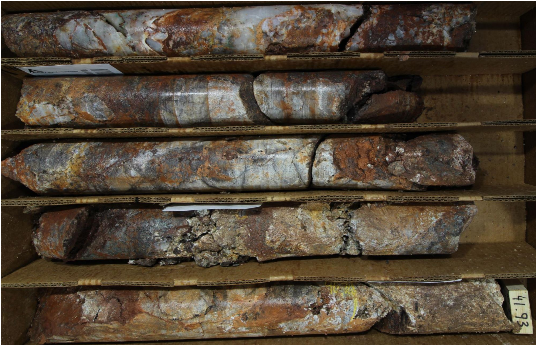
Photo 2. Oxidation of vein sulfide minerals within hematite-diopside skarn zones peripheral to broad quartz veins found in variable intensity within altered limestone host rock at the margins of stockwork-veined quartz dacite porphyry sills in the top 300m of Hole 001 ( Hole 001; 39-42 m interval; HQ ).
