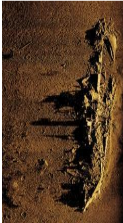
Figure 3: SS Ferrando Shipwreck Imaged by Kraken SAS (courtesy of ECA Robotics)
