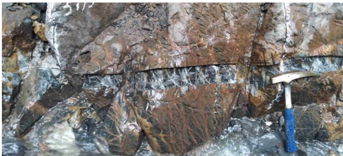
Figure 1. Photo of saw cut channel sample from GUI-CH-002. This style of dense vein stockwork persists to depth and was intersected in Royal Road's previous drilling. This sampled section returned 1.3 grams per tonne gold, 0.5% copper and 6.5 ppm silver.
