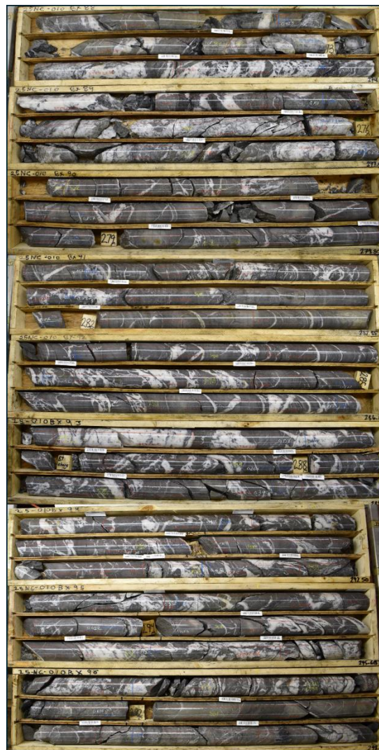
Figure 3. Drill core photos from drill hole 25NC-010 showing a broad intercept of high density narrow sheeted veining hosted in sulphide-mineralized and altered mafic volcanic host rock. Assay results remain pending.
