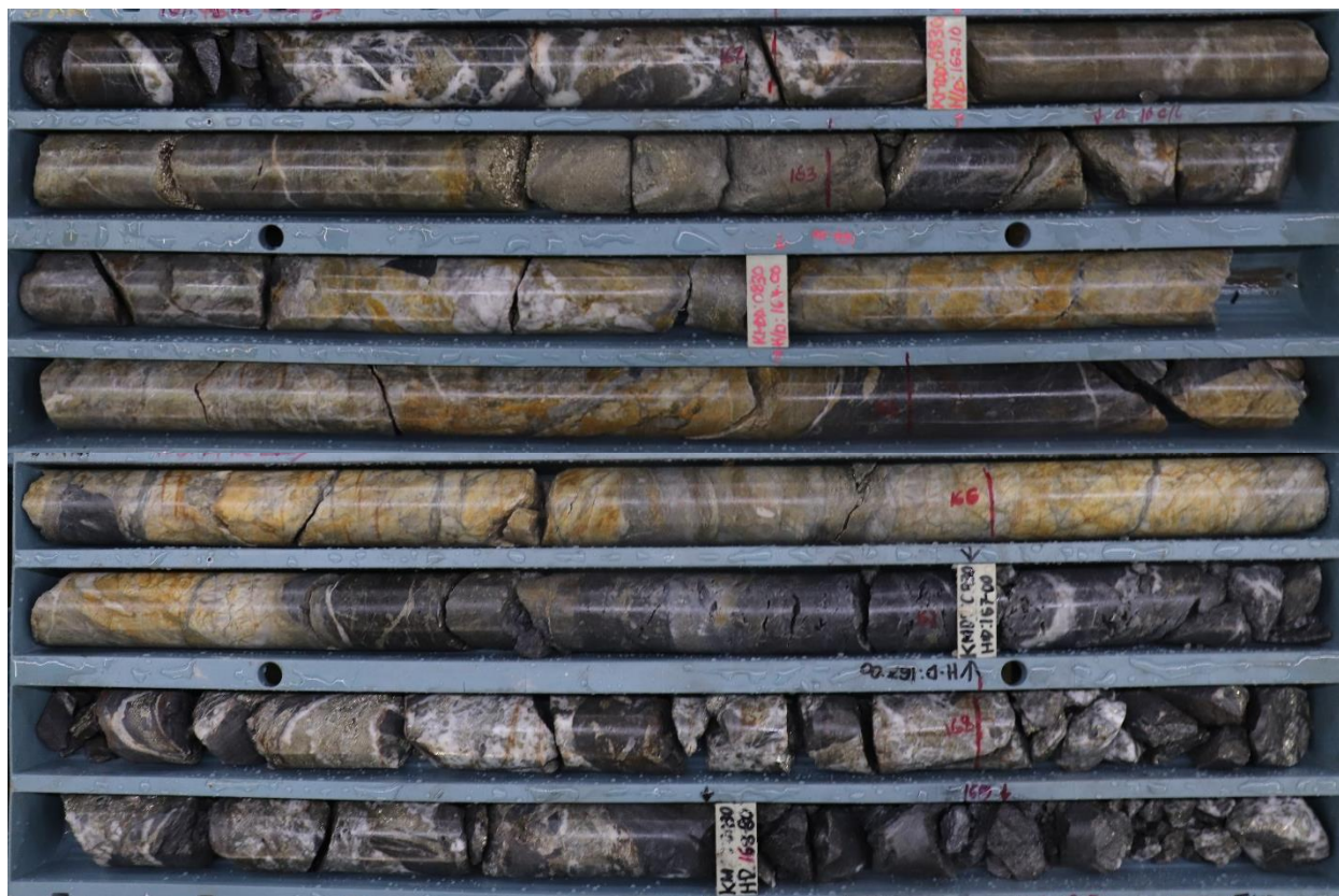
Figure 7 – KMDD0777 Core Photograph, 413.40 – 418.65 m; within intersection of 1.35 m at 23.97 g/t AuEq or 14.38 g/t Au, 147 g/t Ag and 5.04% Cu from the K2 Vein.
