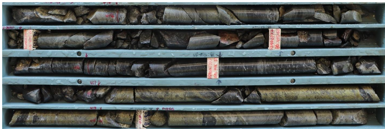
Figure 7 – KMDD0777 Core Photograph, 413.40 – 418.65 m; within intersection of 1.35 m at 23.97 g/t AuEq or 14.38 g/t Au, 147 g/t Ag and 5.04% Cu from the K2 Vein.
