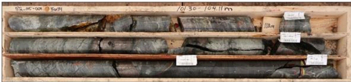
Figure 5 – Hole BR25-004 from 102.0-103.0m containing 1.13% CuEq* within pyroxene-minor garnet skarn with semi-massive bands of pyrrhotite and chalcopyrite.
