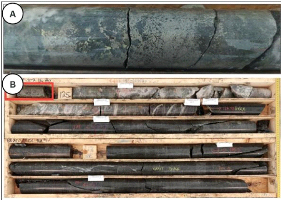
Figure 4 – Hole BR25-002 at 125m. (A) Closeup of massive pyrrhotite > chalcopyrite in skarn zone approaching contact with a thick granodiorite dyke. Interval 124.7- 126.5 contains 1.51% CuEq.
