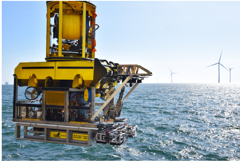
Figure 1: Kraken's Sub-Bottom Imager (SBI) delivers 3D data, enabling a clear understanding of subsea stratigraphy, underwater infrastructure, and hazards.
