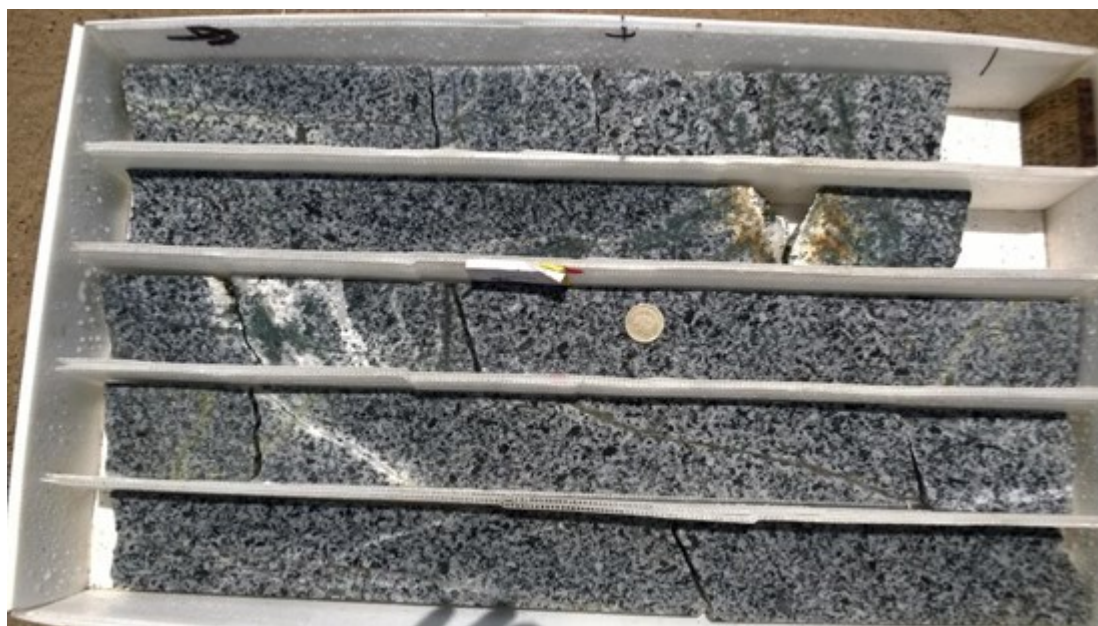
Figure 5: Core from historical drillhole COP14-02 showing quartz veining, copper sulphides and stockwork within granite porphyry. Core shown commences at a depth of 122.85 metres and ends at 125.85 metres. Associated drillhole assay results: 178.7 metres @ 0.23% Cu, 0.022% Mo and 0.9 g/t Ag (from 38.6 metres) (Table 1).
