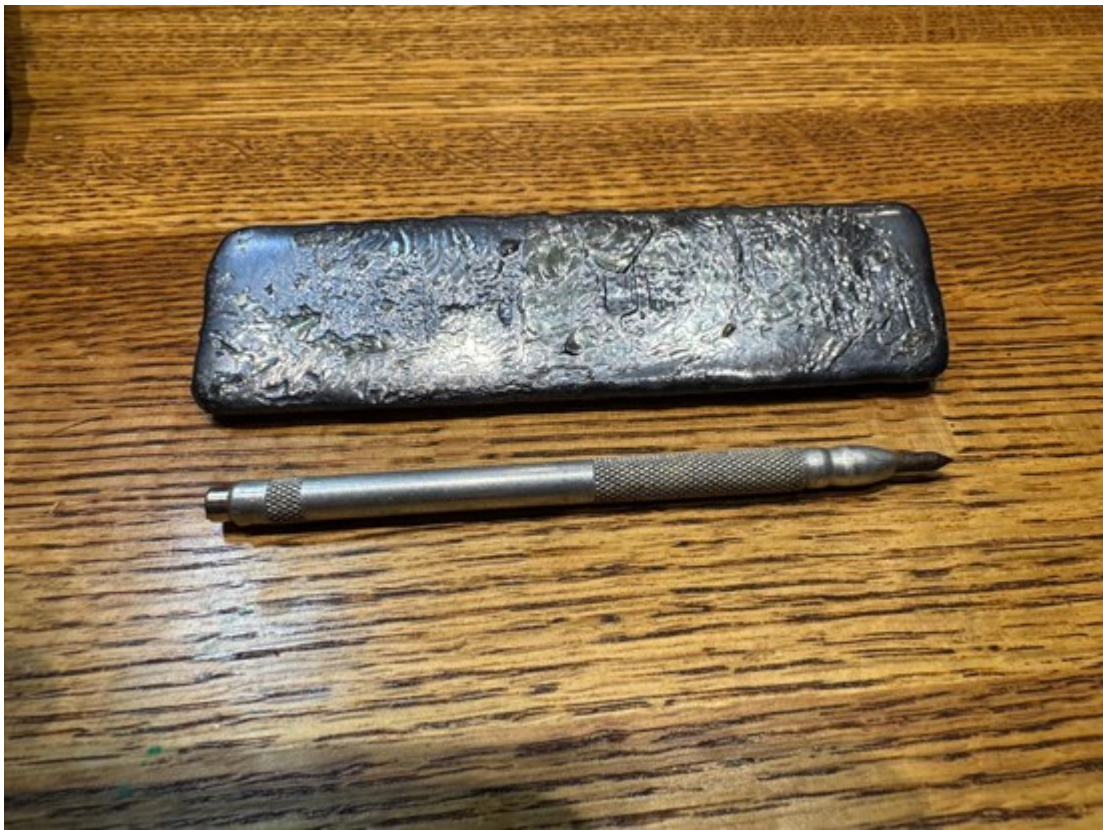
Figure 1: 445-gram (14.3 troy ounce) refined silver bar produced from the Silver Surprise mini-bulk sample via gravity table separation.
