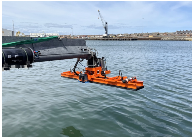
Figure 1: Kraken Robotics' Sub-Bottom Imager (SBI) can be deployed from vessels in nearshore environments, delivering 3D volumetric data down to five meters beneath the seabed.
