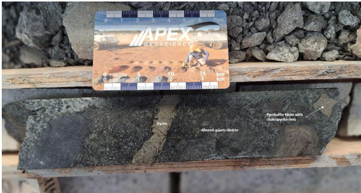
Figure 10: Visual pyrrhotite and chalcopyrite blebs and disseminations within altered quartz-diorite, overprinted by pyrite veining in NQ drill core from approximately 356.95m downhole in drill hole WD26-01. Laboratory assays for this interval are pending.
