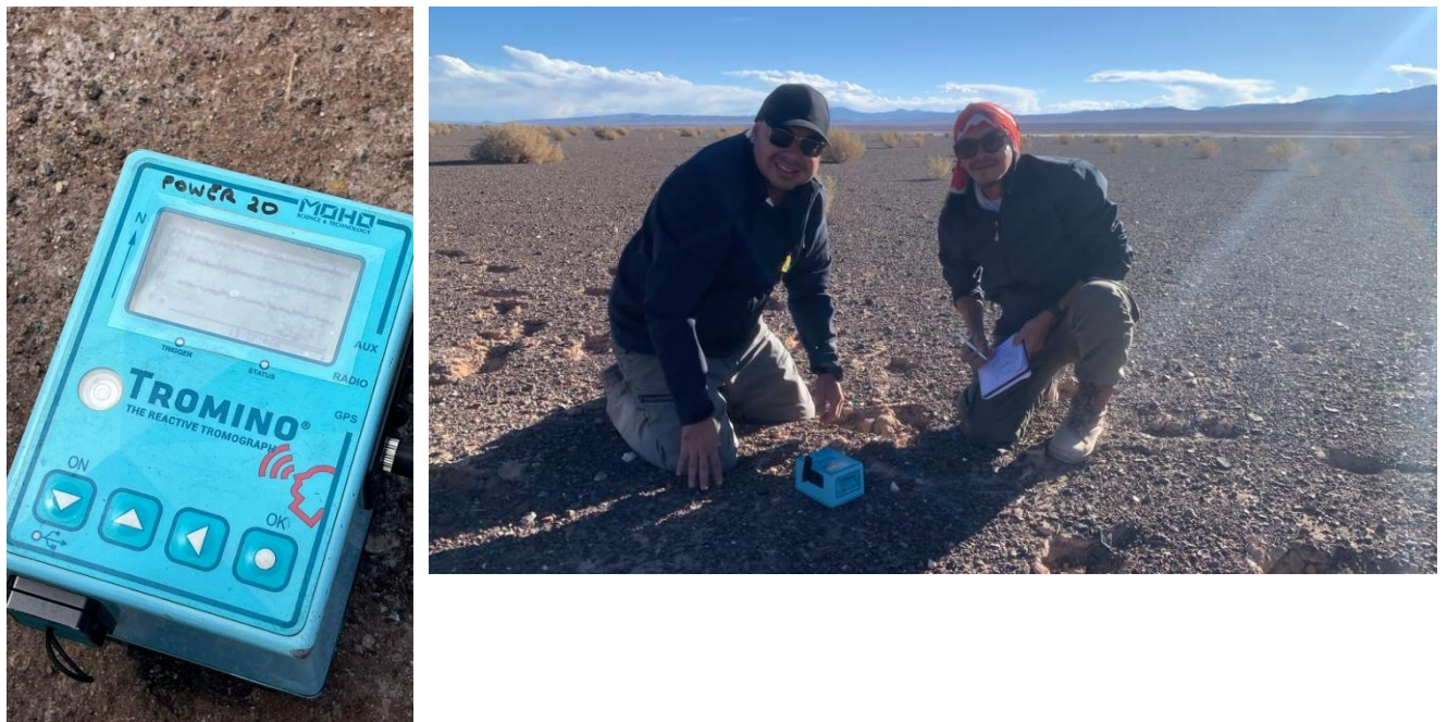
Figure 4: Power field team testing the seismic units on-site at Rincon Lithium Project.
