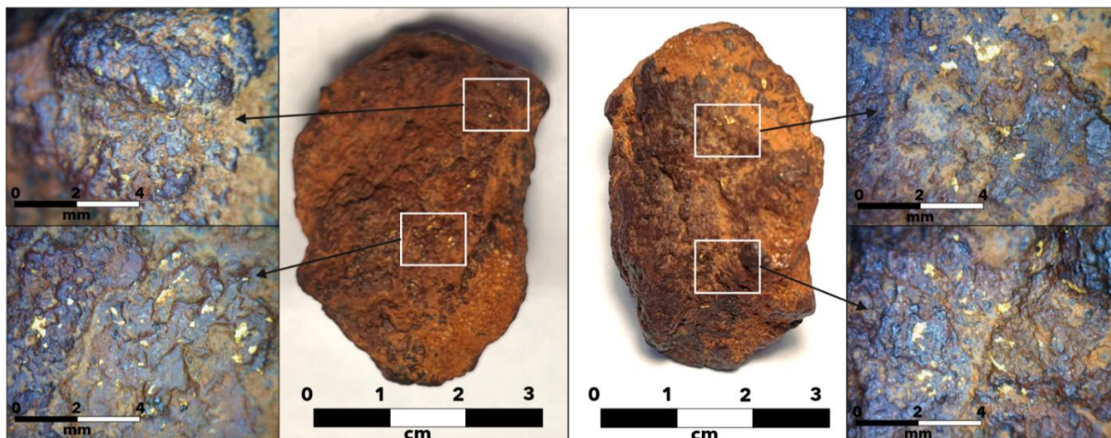
Figure 11: Rock specimen found containing abundant gold at Riverina East Project (268538 East, 6698354 North). Picture shows both sides of the specimen and close up images of showing the gold occurring throughout the sample. Estimated visual abundance of 2-5% Au. Assay required to confirm Au content with results expected in Q1 2026.
