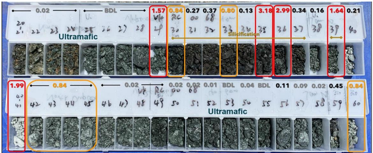
Figure 8: Chip samples from VKRC0068 and analysis results reported as g/t gold. 17m at 1.1g/t Au from 28m with higher grade intercepts up to 3.2g/t as annotated.
