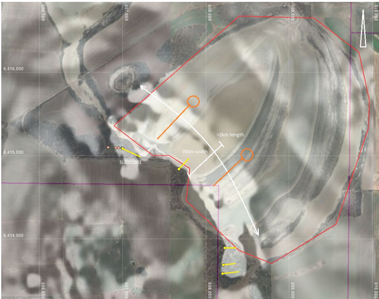
Figure 2: Khal Nickel-Cobalt Project- Plan view of 1VD magnetic signature representing the >2km long, 700m wide ultramafic sequence overlain by aerial photography highlighting the salt lake, with Reserve 18455 (Lot 225568) highlighted in red. Sultan’s 2022 aircore collars are marked in orange, and previous diamond drilling traces in yellow, with recent SLGDD001 named. Orange circles and traces indicate possible drilling collar positions to test the layered intrusion from the salt lake surface.
