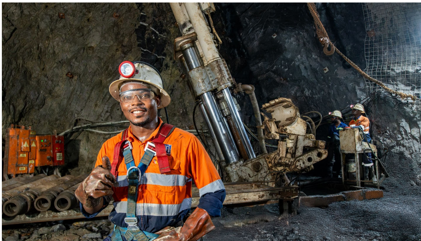
Photo: Raisebore Operator, Progress Chende, drilling the stope slots on the 1,395-metre level.
