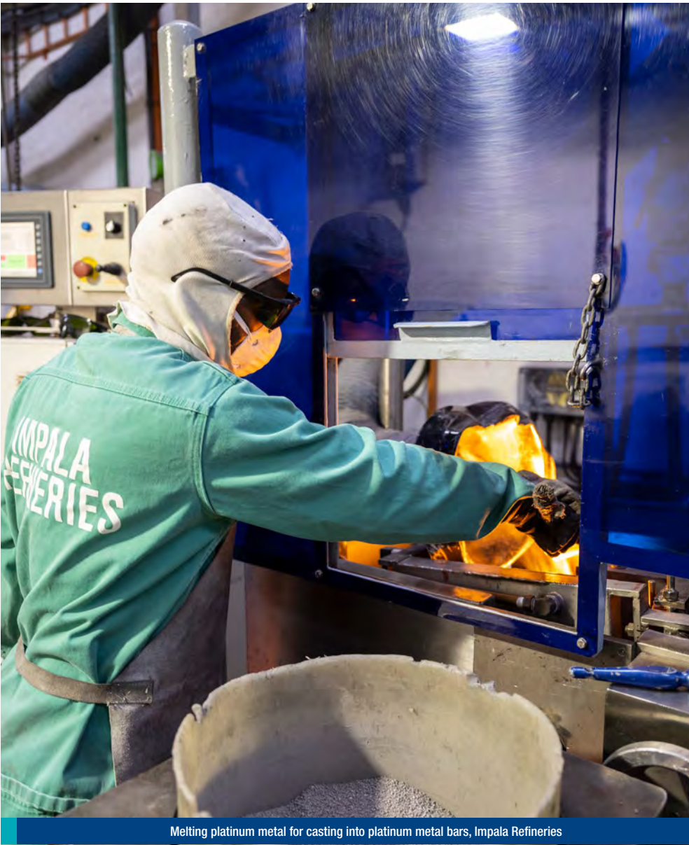
Melting platinum metal for casting into platinum metal bars, Impala Refineries
