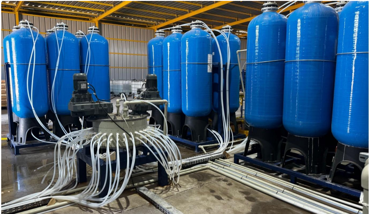
DLE Pilot Plant at R&D Centre in Copiapó, Chile (30 x approx. 3m columns to produce up to 1 tonne per month of LCE)
