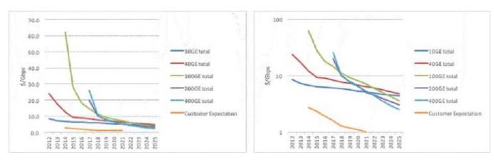
In the above figures that forecast \$/Gbps to 2025 (where the left-hand graph is a linear vertical scale, and the right-hand graph is a log scale), it can be seen that the orange curve plots the customer expectation, while the other color curves show \$/Gbps improvement over time for various high-speed data rate transceivers using PIC based technologies. A gap is appearing between what customer expect and what the technologists can produce.
