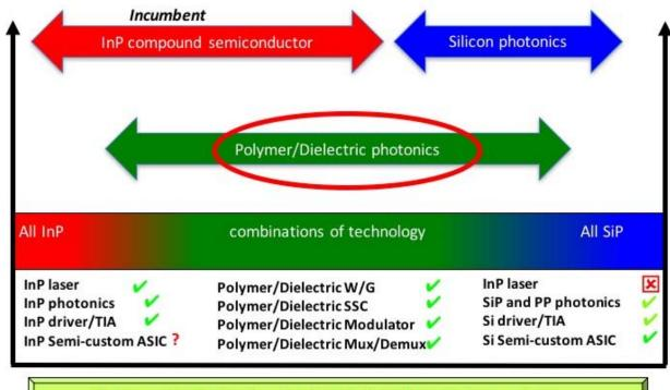
Integrated photonics is critical for datacenters...
