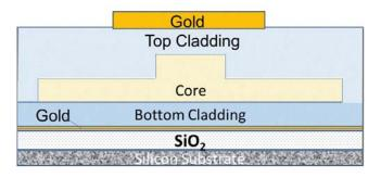
A ridge waveguide modulator is a type of modulator where the waveguide is fabricated within a layer of our electrooptic polymer system. Various cladding materials and electrodes are layered over the core polymer. The polymer materials are then part of an integrated photonics platform that can house other photonic devices, such as lasers, waveguides etc.
