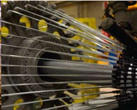
Cable armoring in progress
