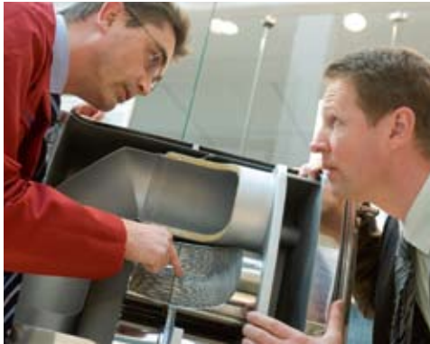
Diesel particulate filter using metal fibers
