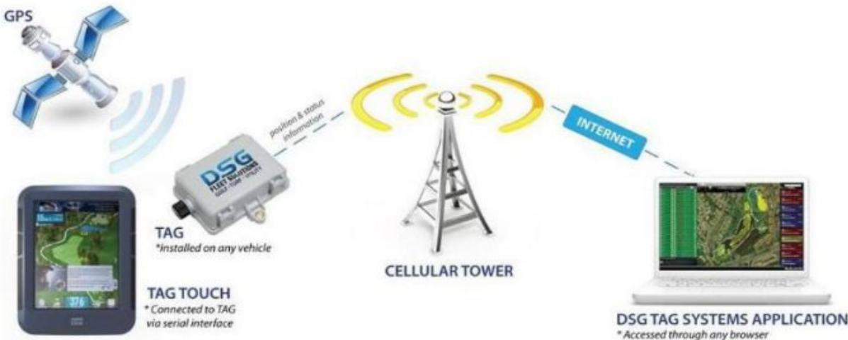
The operator can use the geo-fencing capabilities to create “zones” on the property where they can control the vehicles behavior such as shutting down a vehicle that is entering a sensitive or dangerous area. The TAG System also monitors the strength of the vehicle’s battery helping to prevent sending out vehicles undercharged batteries which can be an inconvenience for the course and negatively impact the golfer experience.
