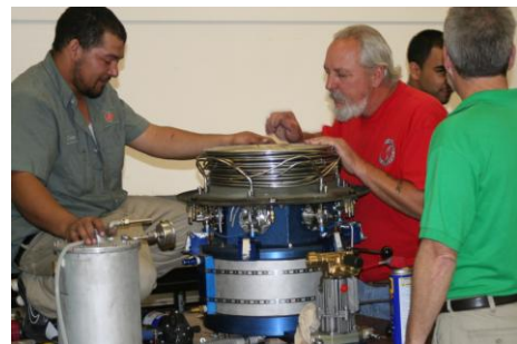
Cyclone technicians preparing the Mark V 100hp engine for test runs – Cyclone received eight patents for this engine in 2010.
