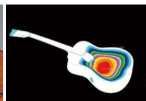
Analysis of the vibrations of guitar surface
