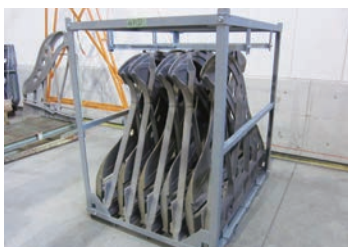
Saving resources and lowering CO 2 emissions by using returnable racks for shipping grand piano frames
