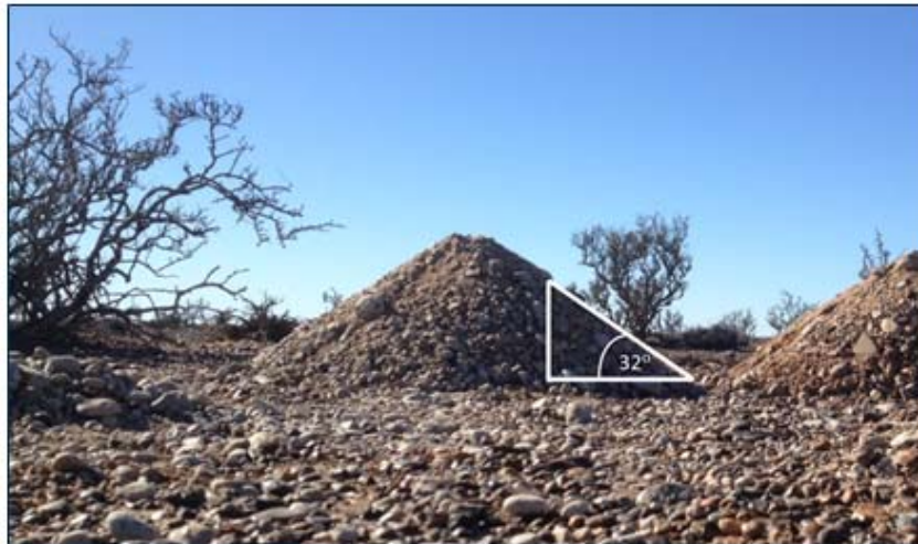
Figure 16-10: Observed angle of repose of dry gravel excavated at Laguna Salada
