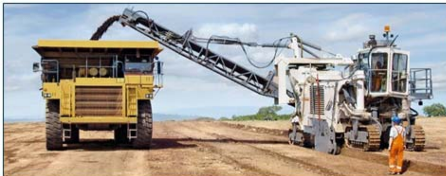
Figure 16-11: Typical operation of a SM 2200 feeding material into a truck via conveyor belt. Source: Wirtgen, 2014
