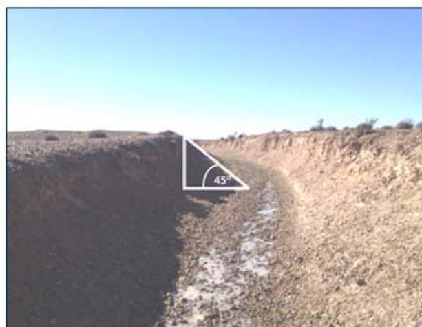
Figure 16-6: Approximately 45° slope angle observed in overburden soil and gravel in the Laguna Salada Project area
