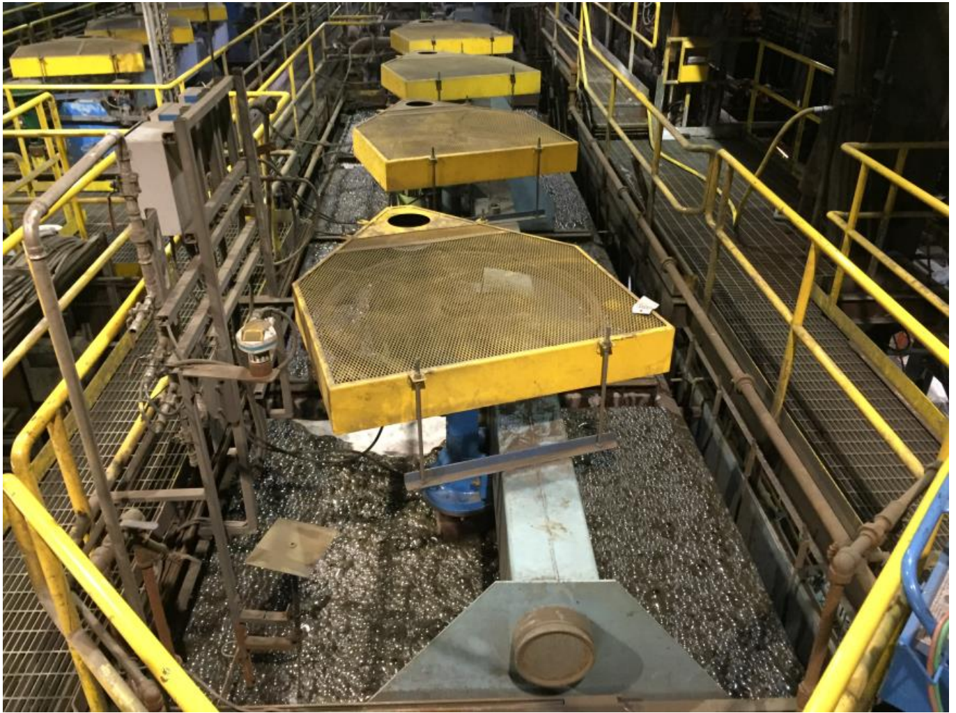
Figure 2: Caribou mill zinc flotation recovery circuit
