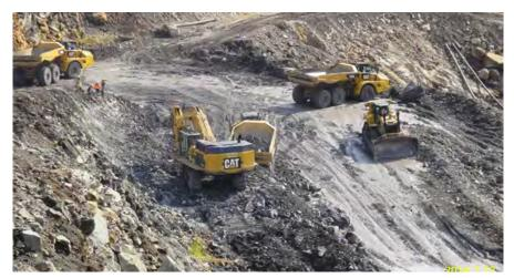
Loading out slope trimming at the ramp from RL-20 to RL-25.
