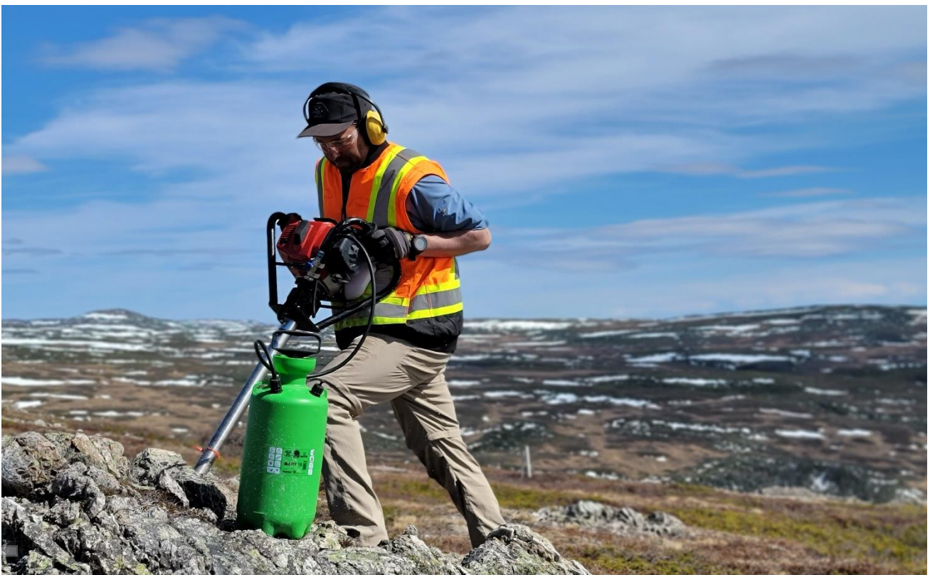
Figure 1: Hand-held power-auger drilling sampling outcrop
