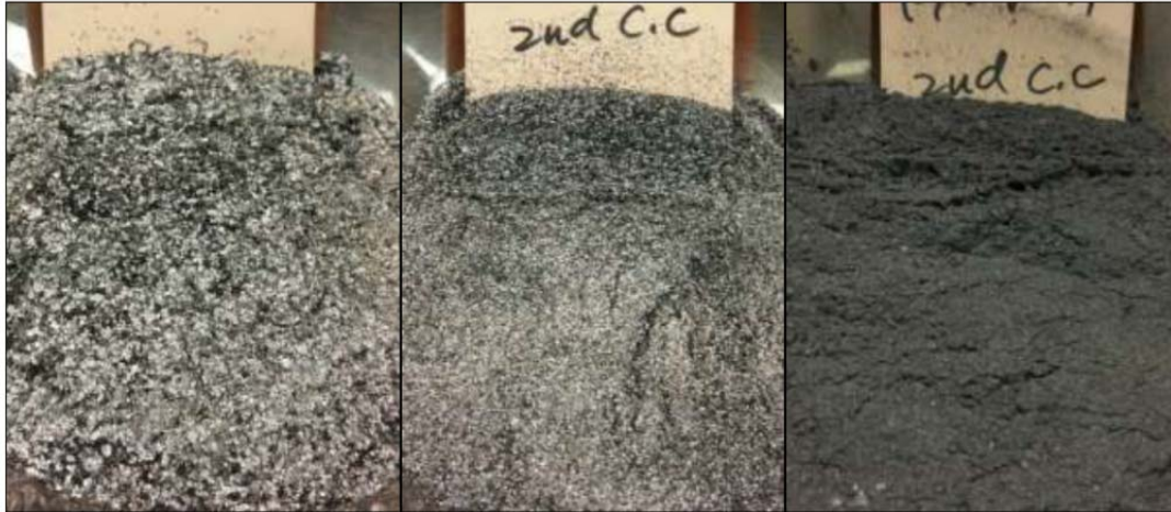
Figure 19: Photograph of +48 mesh (left), +100 mesh (centre) and -100 mesh concentrates
