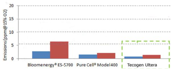
**CHP systems used by EuroSite Power emit significantly less NOx (blue) and CO (red) than other leading systems.**
