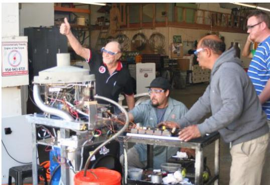
Harry gives the thumbs-up as the Phoenix 10 starts to produce power from waste oil combustion. Phoenix ordered two prototypes in 2010.
