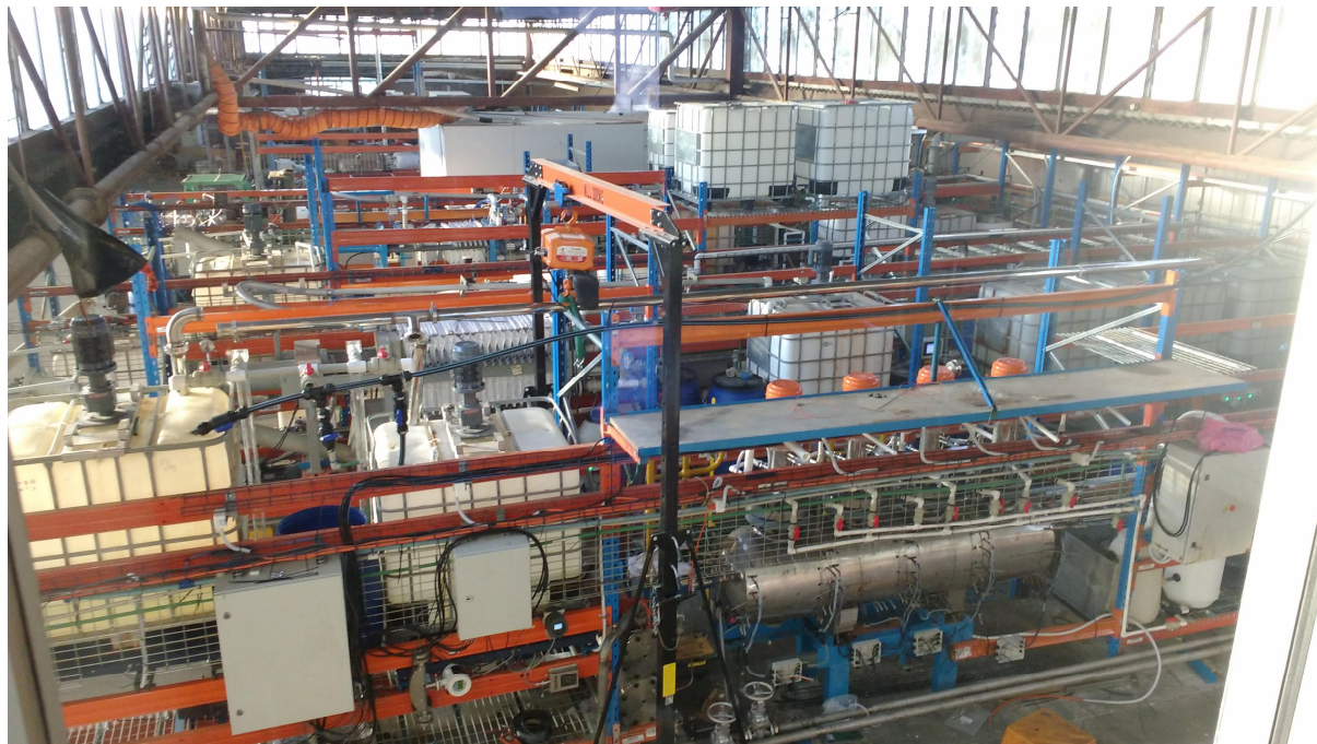
Figure 3: The Demonstration-scale processing plant is a 1:2,500 scale of a commercial 2 million tonne per Pressure Acid Leach + Solvent extraction processing plant. The demonstration-scale plant is located in Simulus Laboratories facilities in Welshpool, Western Australia.
