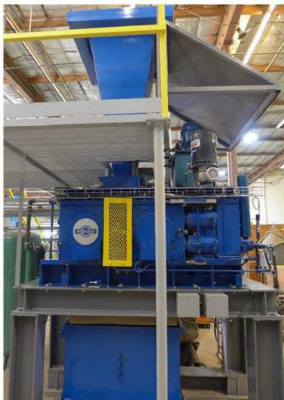
Figure 13.11 View of SMALLWAL HPGR unit at KCA Used for Testing Hasbrouck Samples
