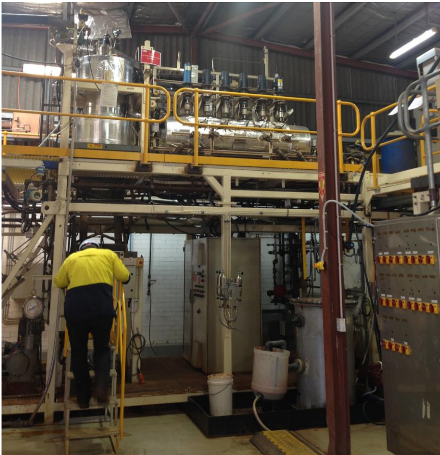
Figure 3: Pilot Plant: High Pressure Acid Leach Autoclave (horizontal cylinder at top of photo)
