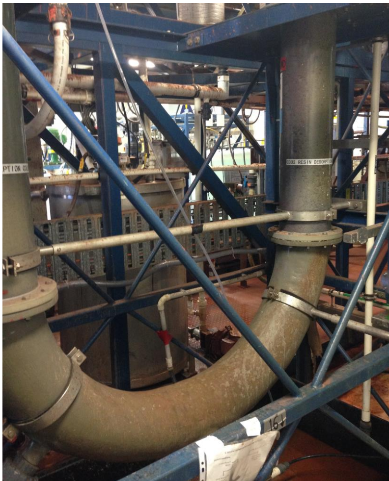
Figure 5: Clean TeQ Pilot Plant: 'U-Column' Nickel/Cobalt Recovery System
