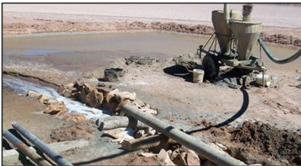
Figure 11.2 Cyclones at RC drilling platform (SRK, 2011)
