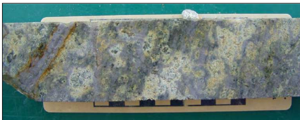
Figure 7.6 B-Type Vein (Left side of core) Cutting Earlier Silicification
