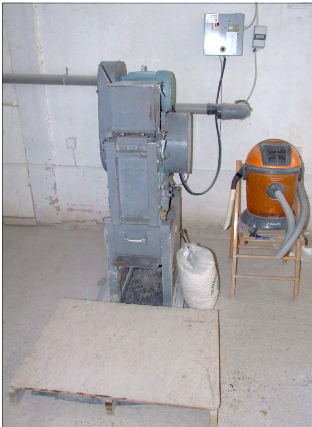
Figure 11.3 Jaw Crusher Equipment at Euromax Resources' Facilities in Strumica
