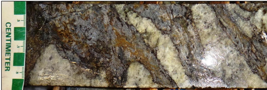
Figure 7-10: High Grade Coarse Graphite in Sheared Pegmatite in Biotite-Graphite Schist (Logged as QGS/QMBGS). From 5 ft. Sample @ 4.56% Cg (ACG-F05, 134 ft.)
