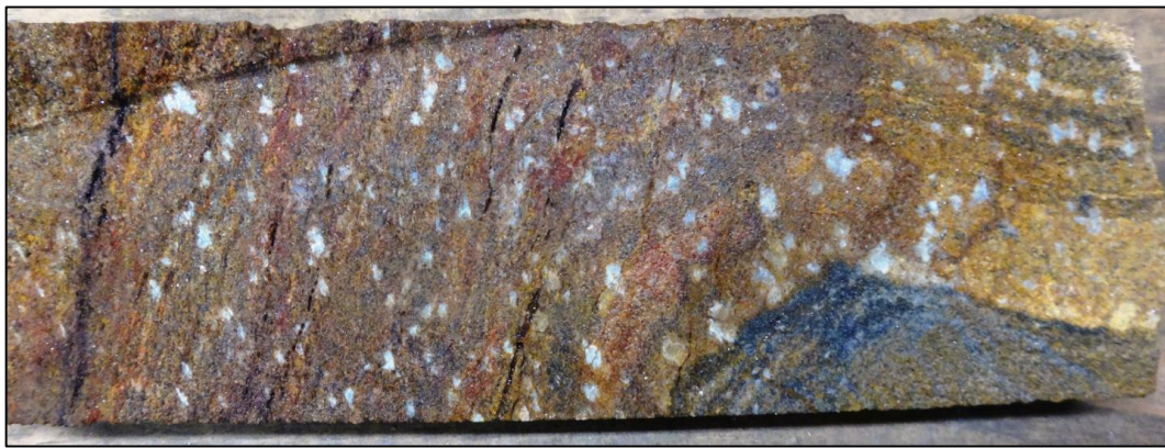
Figure 7-7: Graphite Schist with Green, Vanadium-Rich Muscovite, in the Oxide Zone. From a Sample of 5 ft. @ 2.87% Cg (AGC-15-F15, 24.0 ft.)
