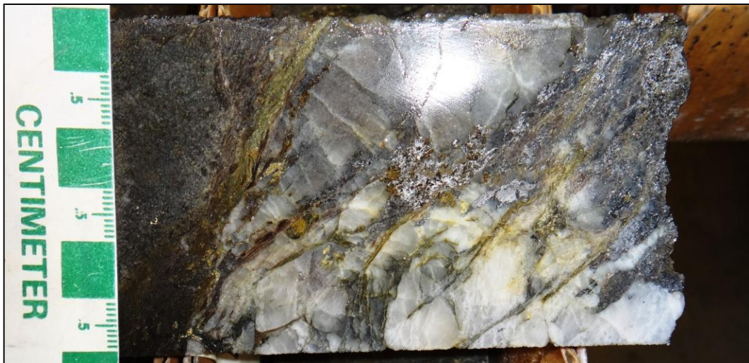
Figure 7-10: High Grade Coarse Graphite in Sheared Pegmatite in Biotite-Graphite Schist (Logged as QGS/QMBGS). From 5 ft. Sample @ 4.56% Cg (ACG-F05, 134 ft.)
