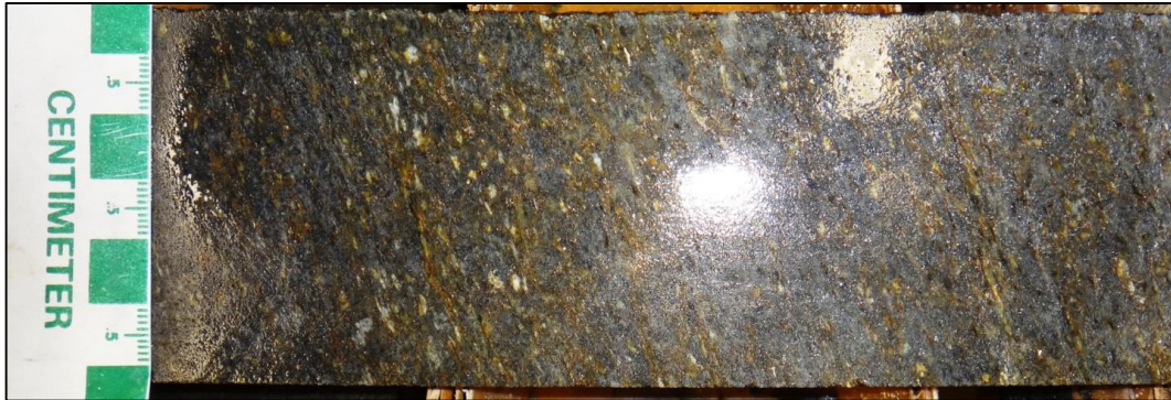
Figure 7-9: Graphite Schist with Folded Pegmatites and Pyrrhotite (Logged as QMBGS). From 5 ft. Sample of 1.73% Cg (AGC-D0, 200 ft.)
