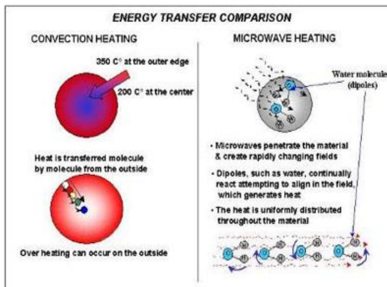
Since water in wet materials usually has a relatively high dielectric loss factor compared to other components, microwave drying can be intrinsically self-regulating. This can lead to the phenomenon of automatic moisture leveling and, ultimately, to efficient drying. Third, microwave energy uses power only when required and is instantly available, making the process suitable for automatic control.
