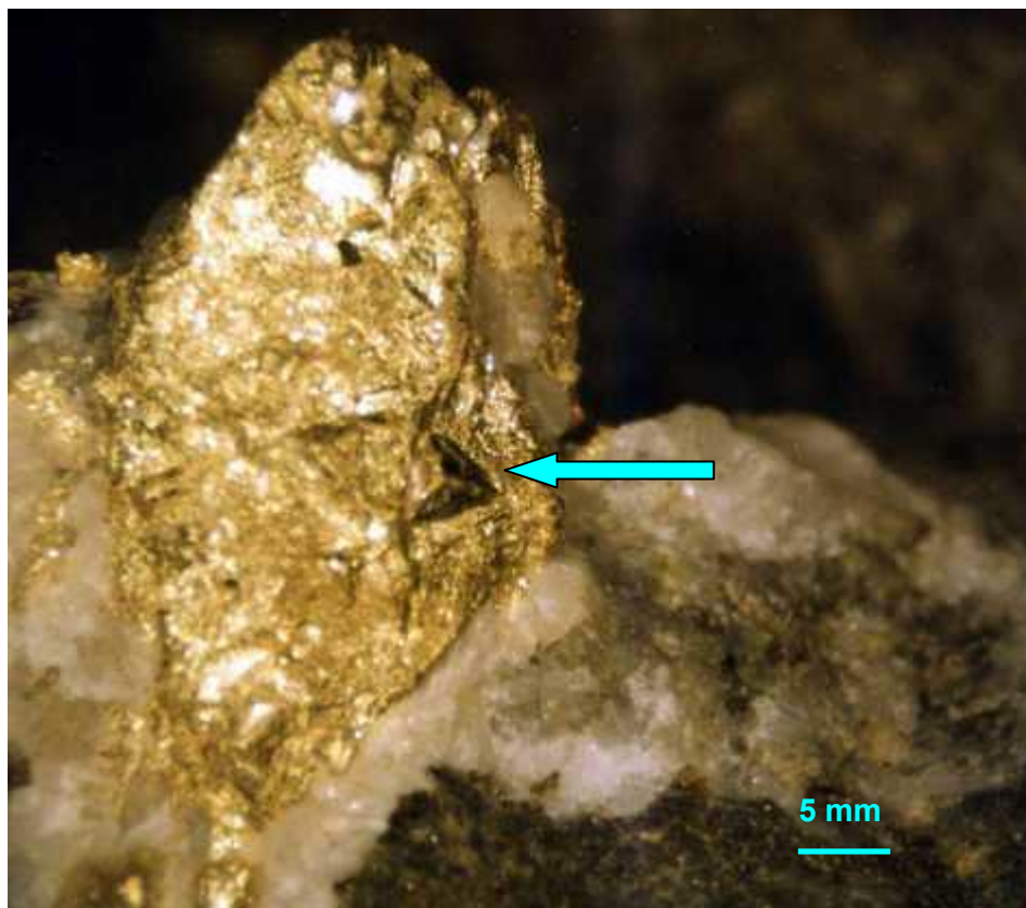
Figure 25: Late stage coarse and partially crystallised gold (shown by arrow) in association with calcite and quartz. Abundancia Vein, Portovelo area (Kalinaj, 2004).
