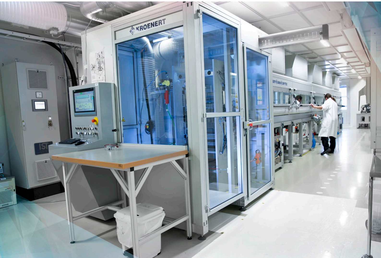
Thinfilm's state-of-the-art, high-volume Kroenert printer has an annual capacity of 50 million integrated systems or 200 million brand protection labels.
