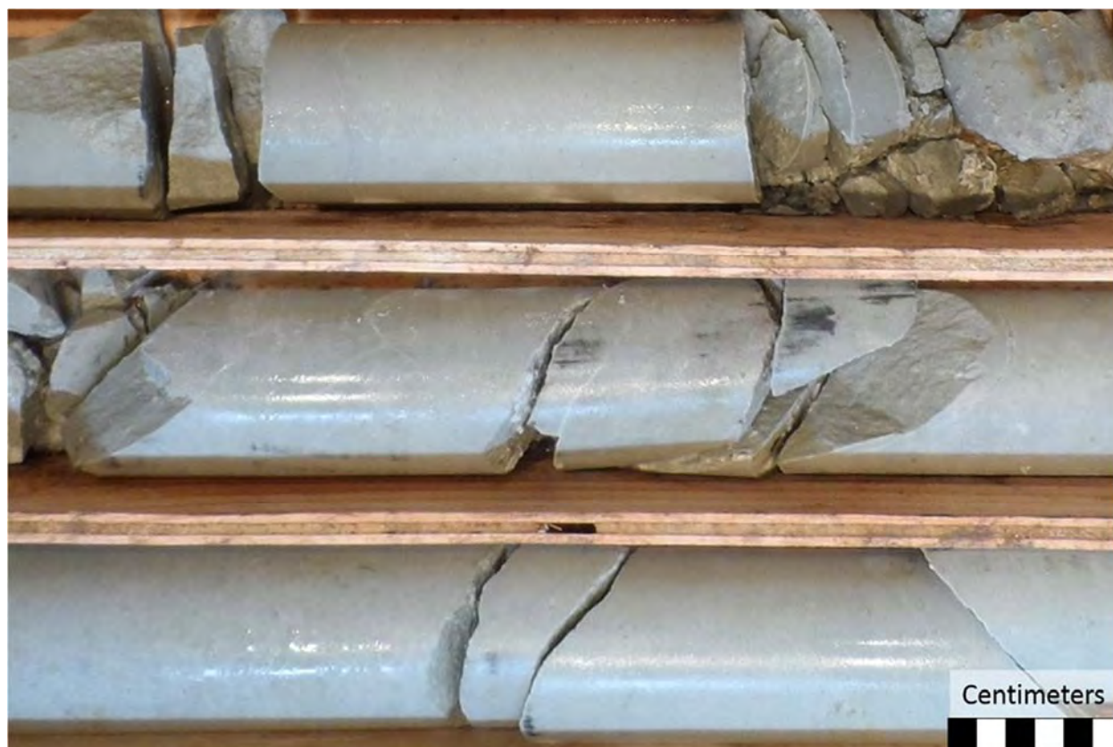
Photograph 7.7: Example of the Rhyolite in HQ Core
