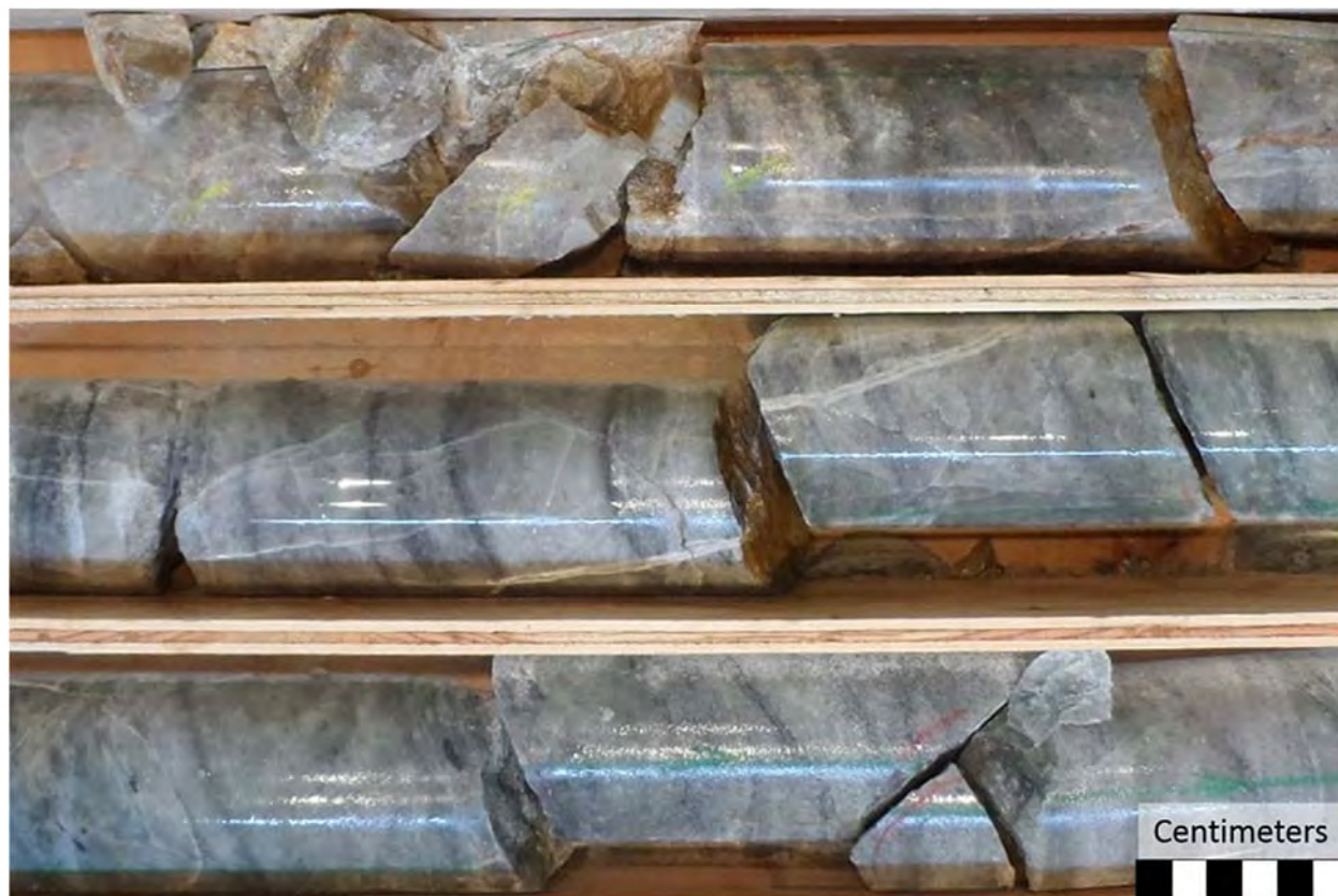
Photograph 7.14: Example of the Lower Quartzite in HQ Core
