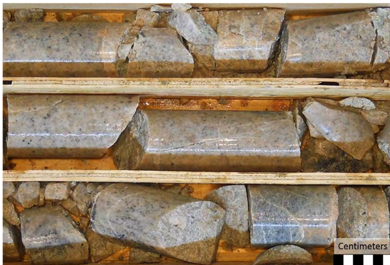
Photograph 7.5: Example of the Granite in HQ Core
