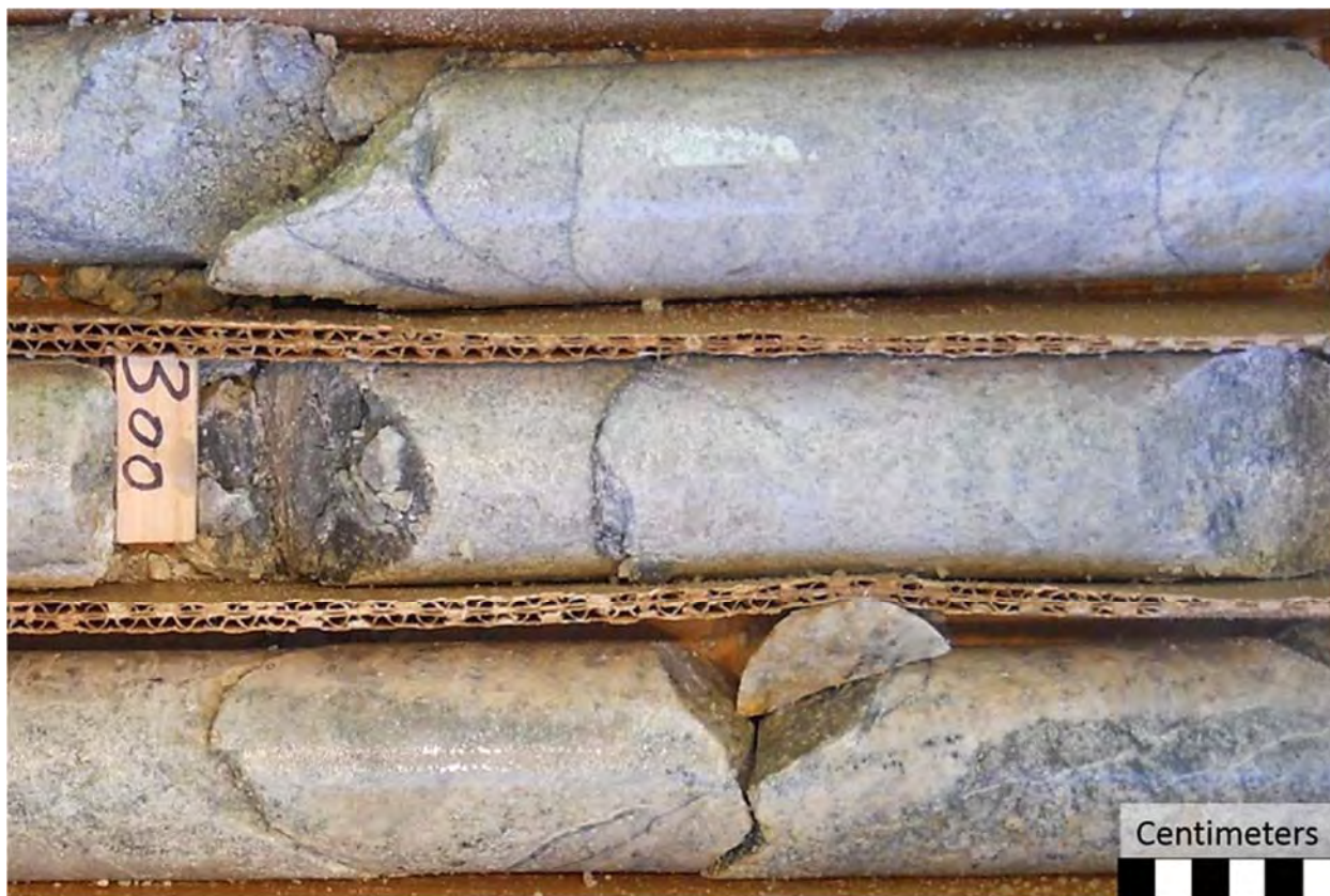
Photograph 7.2: Example of Alaskite in HQ Core
