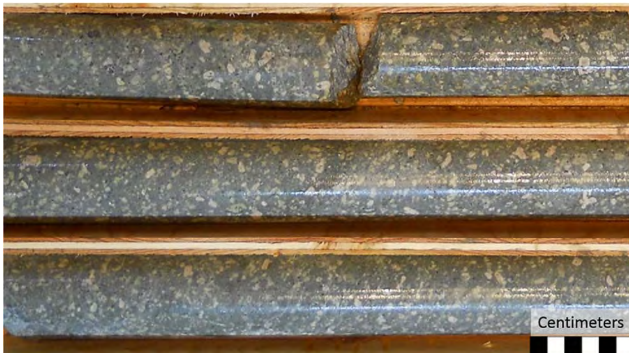
Photograph 7.8: Example of Latite in NQ Core
