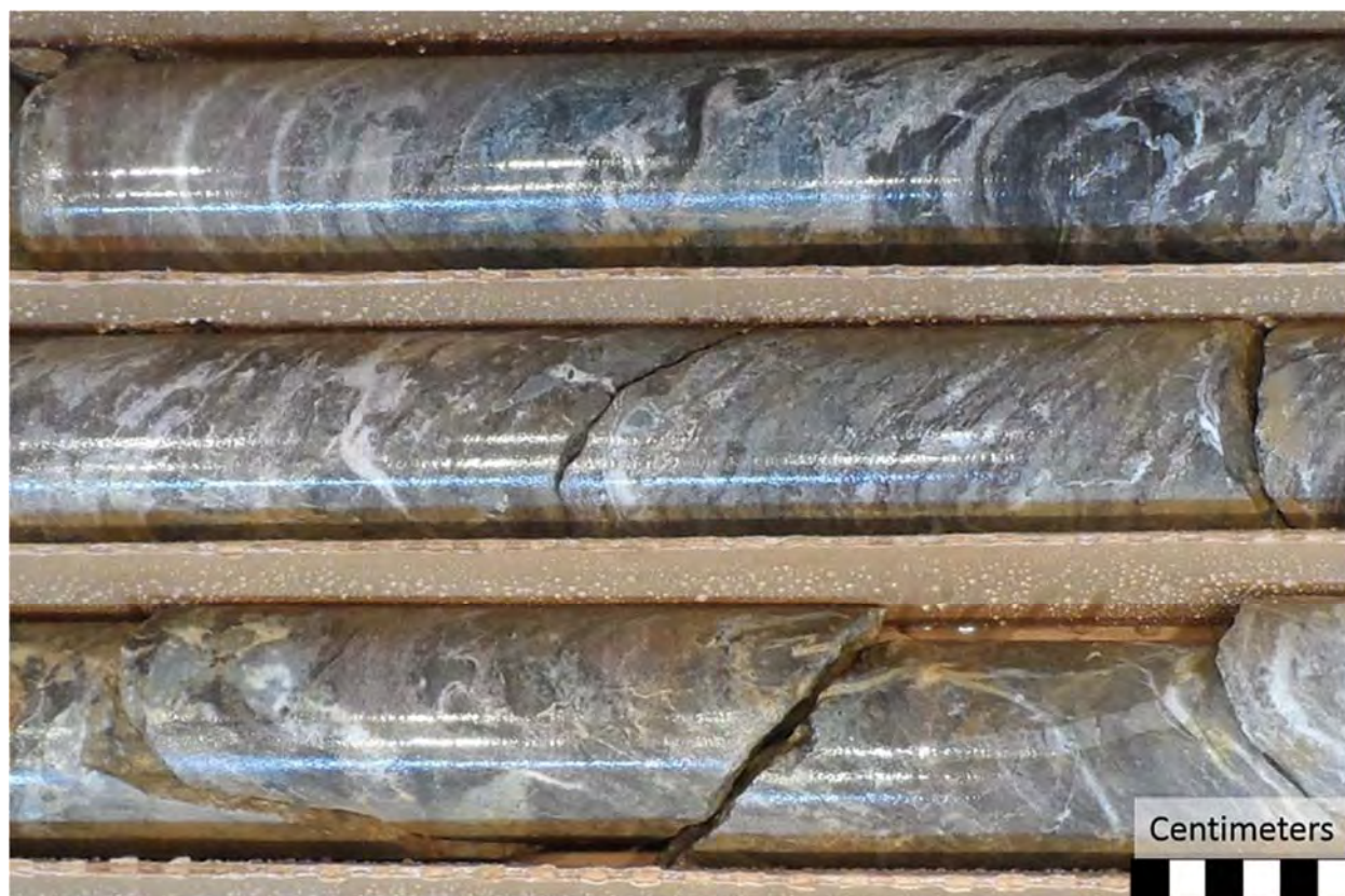
Photograph 7.15: Example of the Upper Calc-Silicate in HQ Core
