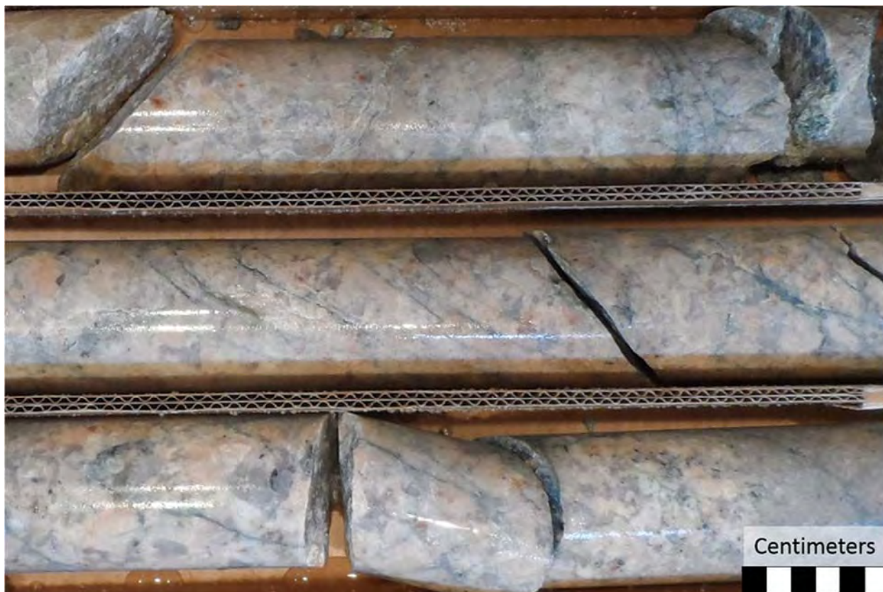
Photograph 7.3: Example of Pegmatite in HQ Core
