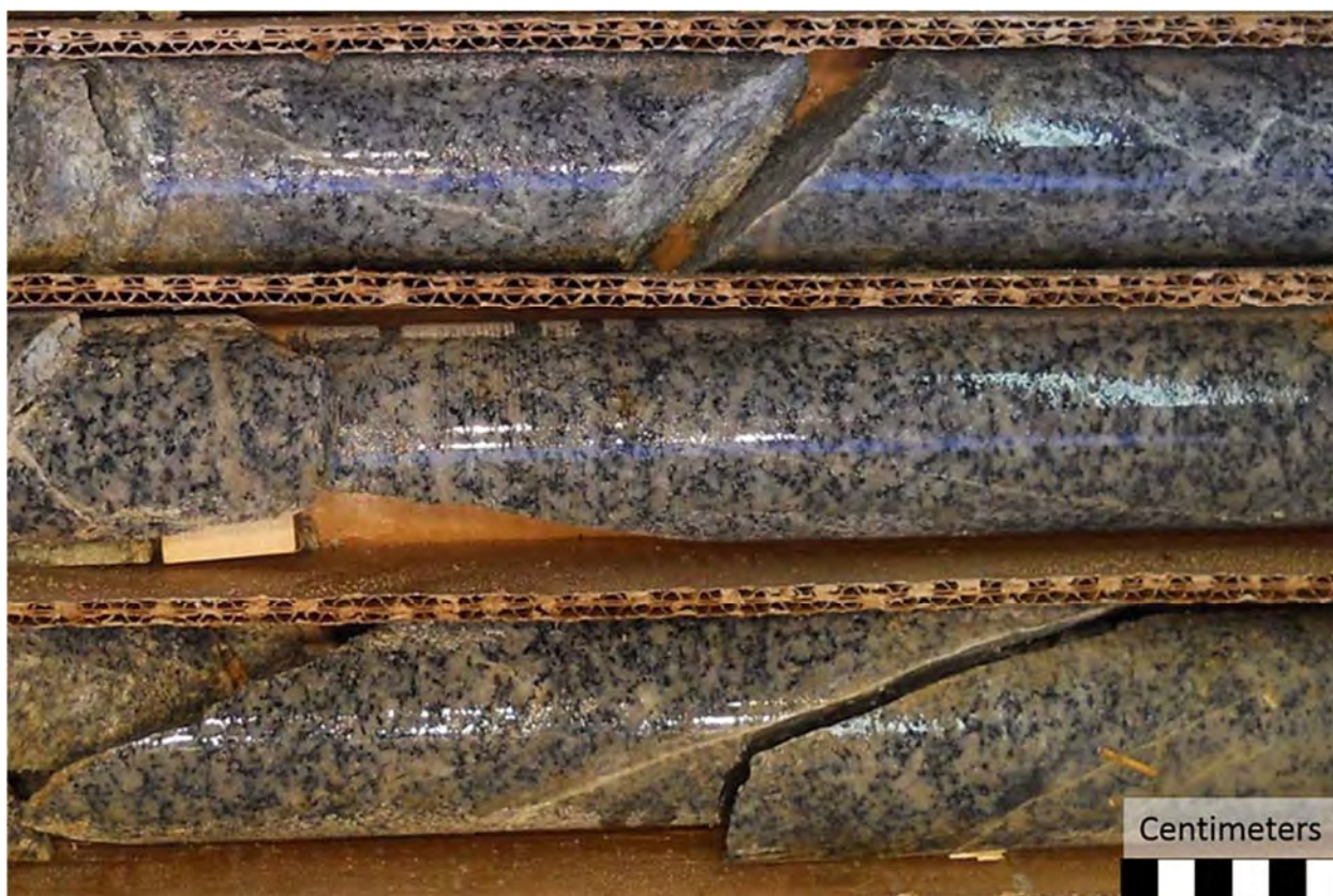
Photograph 7.1: Example of Quartz Monzonite in HQ Core
