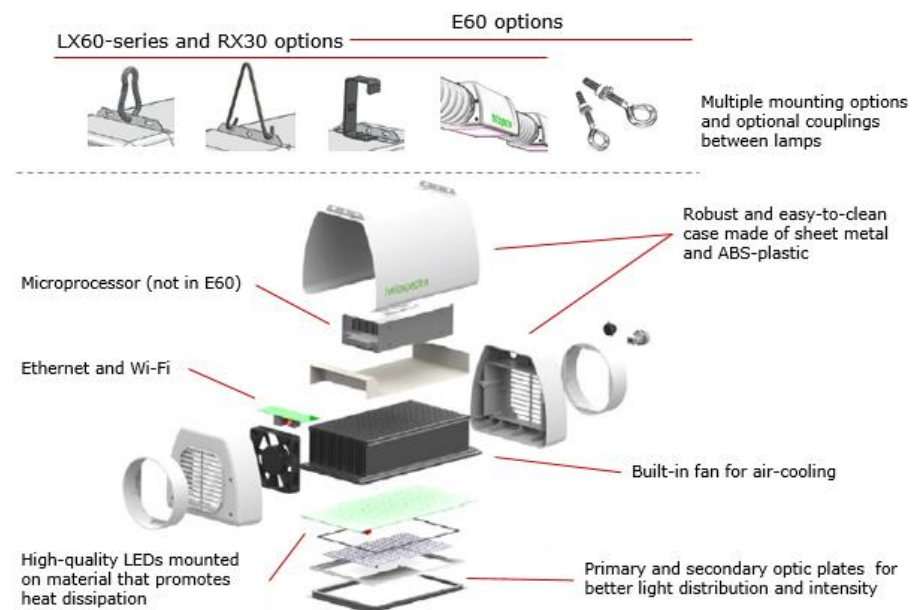
Figure 4: Component break-down of Heliospectra LED grow light (LX60 pictured)
